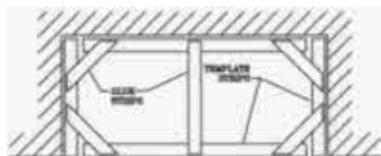
For curved walls or to fit around obstructions you can cut part way thru the template strips and bend it to fit or lay the strips in a spoke fashion to fit to the radius. Again, glue strips on top to hold in place.
